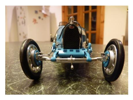
The images above and below show the front axle complete with steering links and leaf spring suspension all operational. The unique positive camber and track of 47.2 inch both front and rear. The type 35 had 94.5-inch wheelbase with a kerb weight of 4,433lbs.
